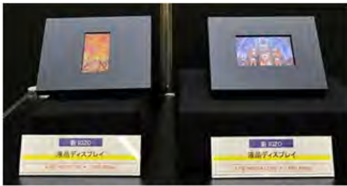
LCD panels incorporating IGZO oxide semiconductor technology
