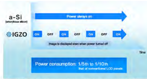
Comparison of energy consumption between Sharp's conventional a-Si LCD panel and the IGZO LCD panel
